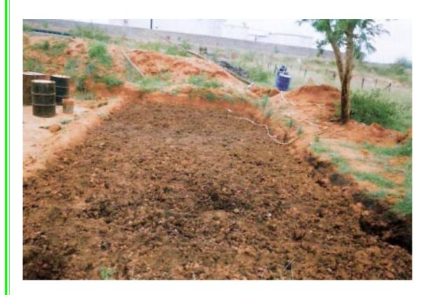
It is noticed that the almost soil like sludge retains water and absorbs it, unlike earlier when water used to slip over the sludge to the sides owing to the nature of hydrocarbons. Now that there are no hydrocarbons left and the sludge got converted to almost like soil, the properties have accordingly changed and the permeability and the porosity of the remediated sludge were akin to that of soil.
