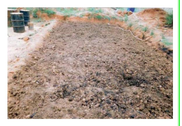
The sludge which underwent two phases of treatment already showed a marked difference in colour and odour. No odour was traceable and top colour was changed to almost like soil. The consistency of the sludge also was changed. The sludge became breakable with fingers unlike earlier, which was soggy.
